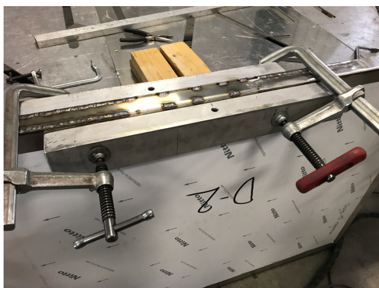
The rig and bracing used in a flawed test to use 2mm stainless steel and avoid canning of the metal surface
